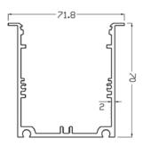
Suitable for two T5, T 8 Lighting tubes or Led Strips.
