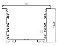
Suitable for two T5, T 8 Lighting tubes or Led Stips.
