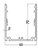
Suitable for two T5, T 8 Lighting tubes or Led Strips.
