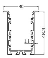
Suitable for one T5 Lighting tube or Led strips.
