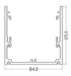
Suitable for two T5, T 8 Lighting tubes or Led Strips.
