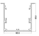
Suitable for two T5, T 8 Lighting tubes or Led Strips.
